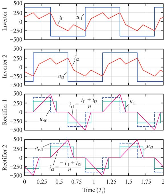
Fig. 10. Simulated primary- and secondary-side voltage and current waveforms of the CISABC according to Fig. 7 with turns ratio  $n = 1$  (no-load rectifier voltage shown dashed), total leakage inductance referred to the secondary side  $L_{\text{os,tot}} = 1 \mu\text{H}$ , switching frequency  $f_s = 50 \text{ kHz}$ , input voltage  $U_i = 800 \text{ V}$ , output voltage  $U_o = 600 \text{ V}$  and duty cycle  $d = 0.5$ .
