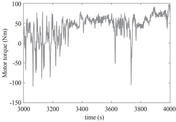
Fig. 2. Dynamic torque request corresponding to the driving cycle of Fig. 1.
