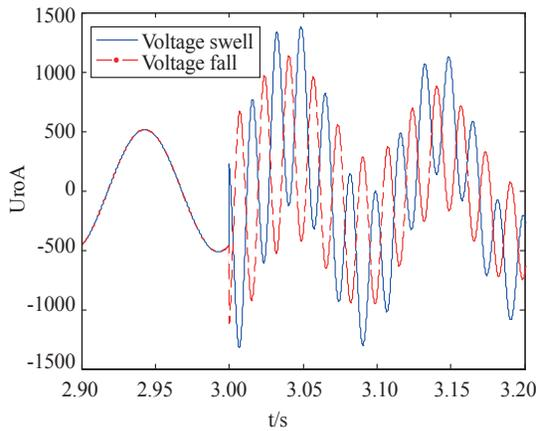
Fig. 4. A phase voltage of rotor in power grid failure.
