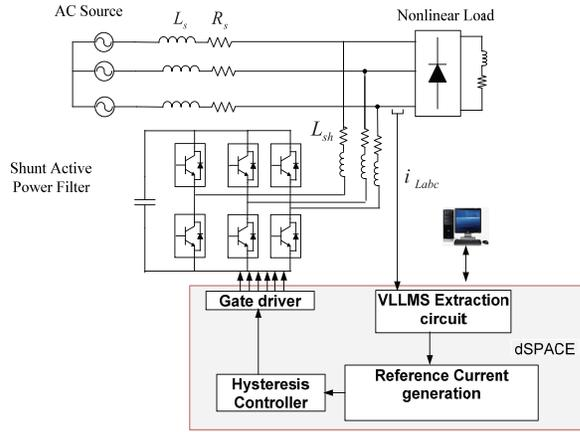
Fig. 10. Block diagram of experimental prototype compensation.
