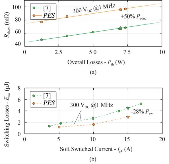
Fig. 15. Comparison between  $R_{TCM}$  (orange) and  $R_{DC}$  (green) as function of  $P_{th}$  (a). The online measurement of conduction losses enabled by the proposed OVMC, more representative of the real operating conditions, results in higher (i.e.  $\approx 50\%$ )  $P_{cond}$ . The mismatch results in lower estimated  $P_{sw}$  (i.e.  $\approx -28\%$ ) according to the calculation reported in TABLE III (b).
