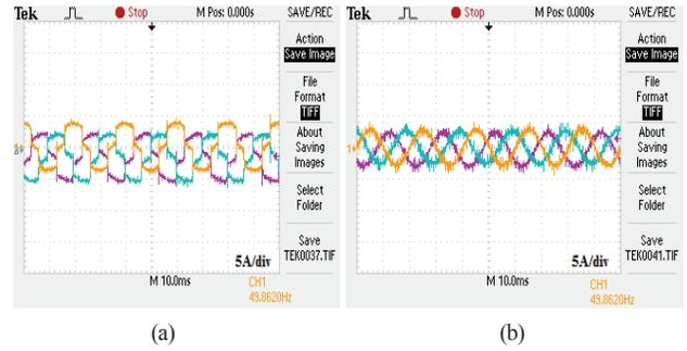
Fig. 12. Nonlinear load and unbalance linear load case (a) Load current, (b) Source current after compensation.
