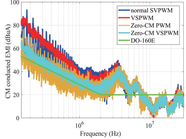
Fig. 28. Comparison of CM conducted EMI (experimental result).
