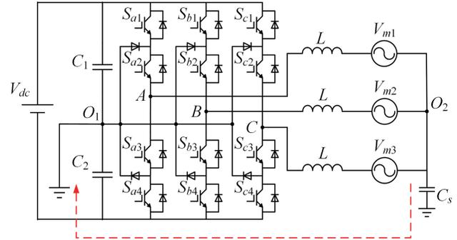
Fig. 1. Topology of three-level NPC inverter.
