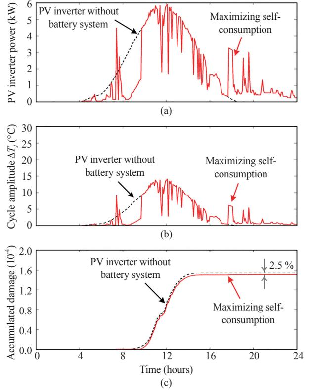
Fig. 8. Loading of the PV inverter with the maximizing self-consumption control strategy: (a) PV inverter power  $P_{pv}$ , (b) the thermal cycle amplitude of the power device  $\Delta T_j$ , and (c) the damage accumulation of the power device.
