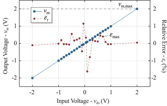
Fig. 6. Results of the DC calibration of the proposed OVMC. When a DC voltage  $-2\text{ V} < v_{ds} < 2\text{ V}$  is applied at the input (x-axis), the output  $v_m$  (left y-axis) deviates less than 5 mV, corresponding to  $\epsilon_r < 2\%$  (right y-axis) in worst-case.
