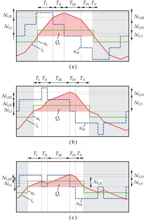
Fig. 13. Rectifier current, rectifier voltage and rectifier no-load voltage waveforms of the CISABC for CCM1 in working point D of Fig. 14(a), CCM2 in working point E of Fig. 14(b), CCM3 in working point F of Fig. 14(c).
