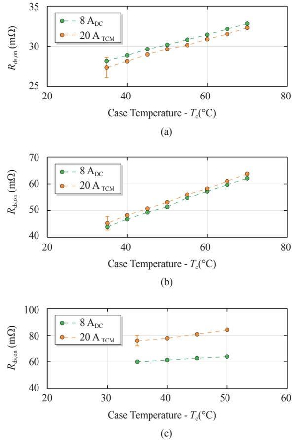
Fig. 14. Average value of  $r_{ds,on}$  measured with the proposed OVMC for different operating conditions of the half-bridge, for different DUTs (TABLE II) and as a function of  $T_c$ .  $R_{TCM}$  (orange) and  $R_{DC}$  (green) are similar (within  $\pm 5\%$ ) for Specimen A (a) and B (b) when the power loss conditions are matched. In the case of Specimen C, a significant discrepancy (i.e.  $\approx 50\%$ ) between the two measurement sets is observed (c).
