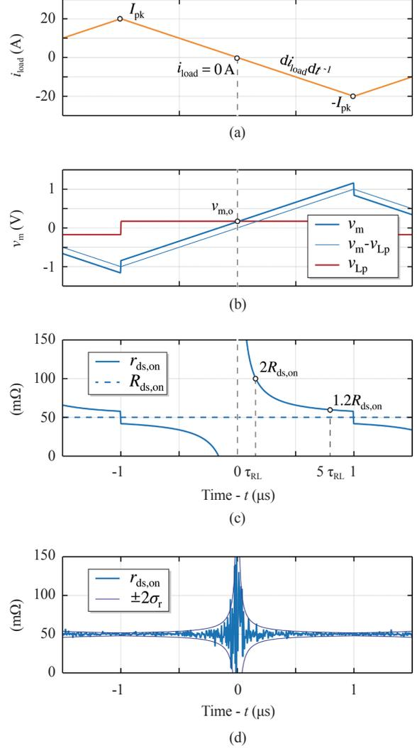
Fig. 12. Comparison of real and ideal waveforms simulated on the half-bridge (Fig. 1) operating in TCM. The combination of  $L_P$  and  $di_{sw}/dt$  causes a distortion on  $v_m$  (b) and consequently on  $r_{ds,on}$  (c). Moreover, a measurement error on  $v_m$  translates into an error on  $r_{ds,on}$  (d) according to (16), particularly amplified for small  $i_{sw}$ , as in (15).
