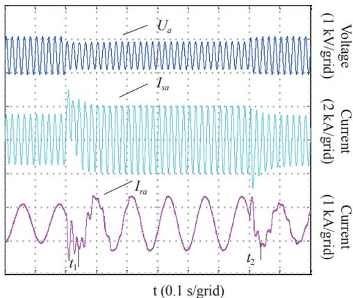
(a) Experimental waveforms for DFIG current and voltage when the grid voltage drop to 70%.
