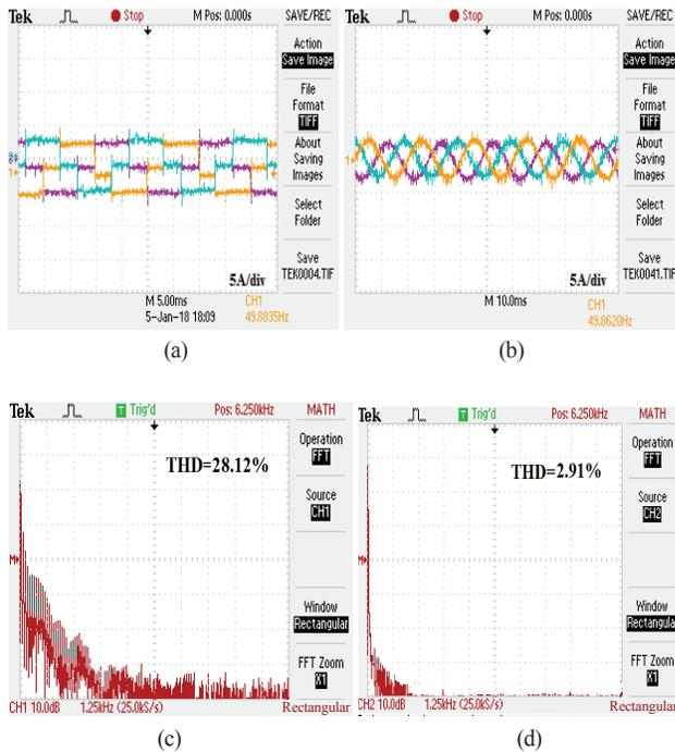
Fig. 11. Nonlinear load case (a) Load current, (b) Source current after compensation, (c) THD before compensation of load current, (d) THD after compensation source current.
