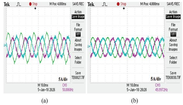
Fig. 13. Unbalance linear load case (a) Load current, (b) Source current after compensation.
