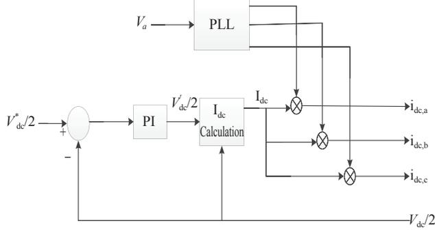
Fig. 3. Three phase self-charging circuit with PI controller.
