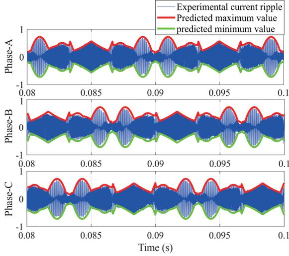
Fig. 7. Current ripple comparison between experiment and prediction (Normal SVPWM).
