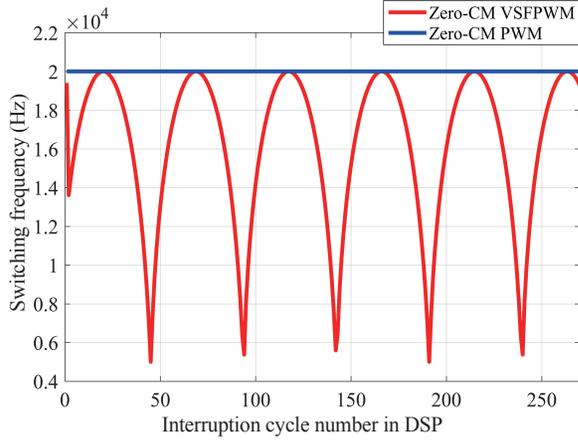
Fig. 26. Switching frequency variation of zero-CM VSFPWM in DSP .
