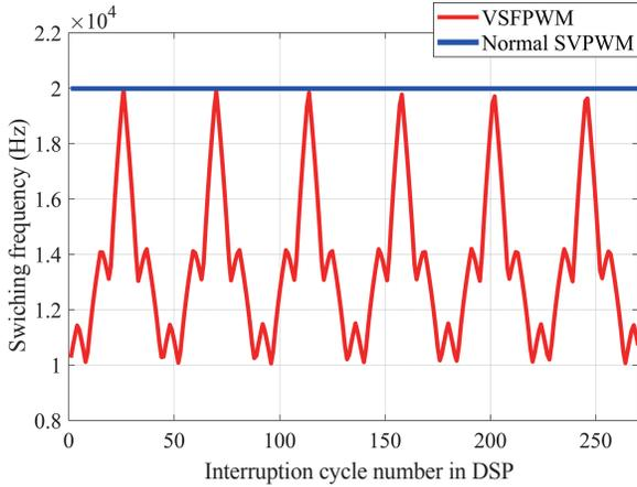
Fig. 10. Switching frequency variation of VSFPWM (experimental result).
