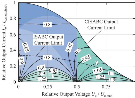
Fig. 15. RMS inverter current to DC output current ratio of the CISABC and output current limit compared to the output current limit of the ISABC.
