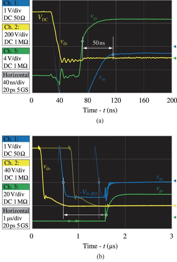
Fig. 10. Analysis of the dynamic response of the proposed OVMC. (a) less than 50 ns after  $v_{gs}$  has reached  $V_{th,T_2}$  (green dot),  $v_m$  (blue) is settled to the correct value, even in the case of significant  $V_{fv,BD}$ , e.g.  $> 2$  V. (b) when  $V_{fv,BD}$  is in the measurable range, the proposed OVMC allows to monitor the conduction time of  $D_{T_2}$ , evaluating the dead-time conduction losses and its effective duration.
