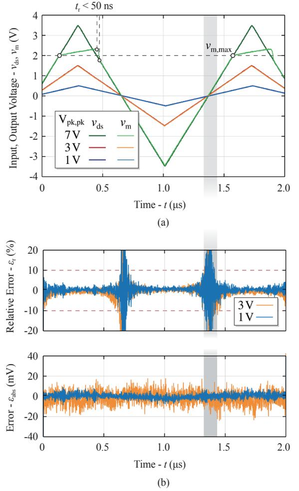
Fig. 7. Results of the AC calibration of the proposed OVMC. When AC voltage waveforms of different amplitudes are applied at the input  $v_{ds}$ , the output waveforms  $v_m$  are practically indistinguishable from them:  $\epsilon_{abs}$  is limited by the oscilloscope resolution.
