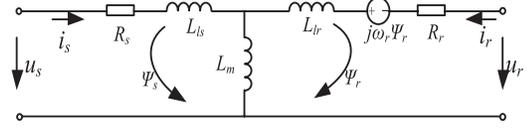
Fig. 1. Equivalent circuit of DFIG.
