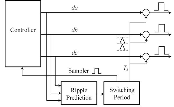
Fig. 8. Structure of VSFPWM generation.
