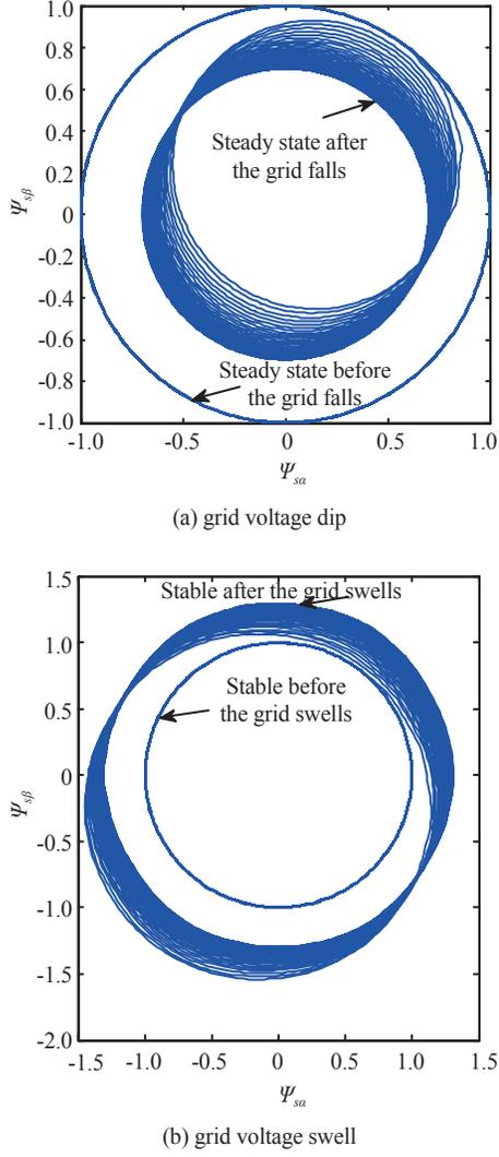
Fig. 2. Stator flux waveforms in  $\alpha\beta$  frames during grid voltage fault.
