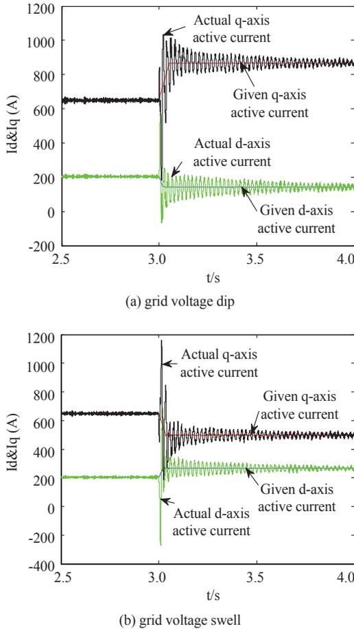
Fig. 7. Rotor current in dq frame with 30% change in grid voltage amplitude.
