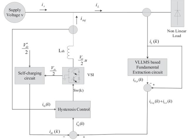
Fig. 1. System block diagram of single-phase adaptive shunt active filter.
