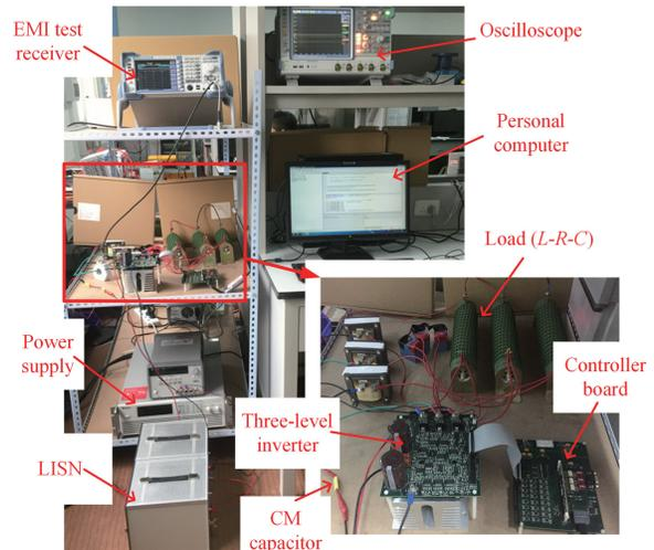
Fig. 2. Experimental platform.
