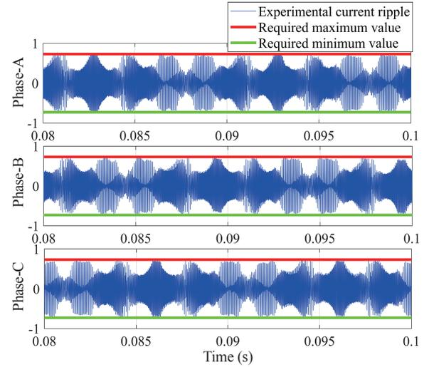
Fig. 9. Three-phase current ripple of VSFPWM (experimental result).
