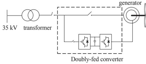
Fig. 6. Experiment and simulation structure diagram of DFIG.
