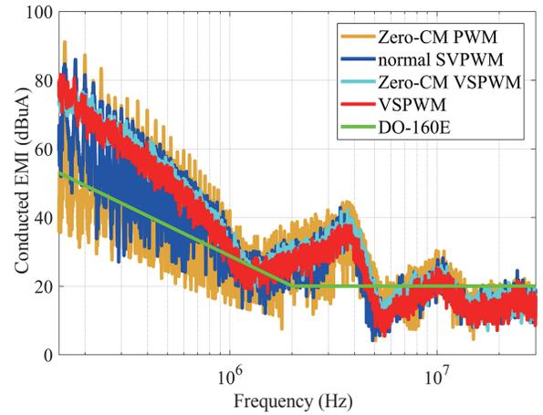
Fig. 29. Comparison of conducted EMI (experimental result).
