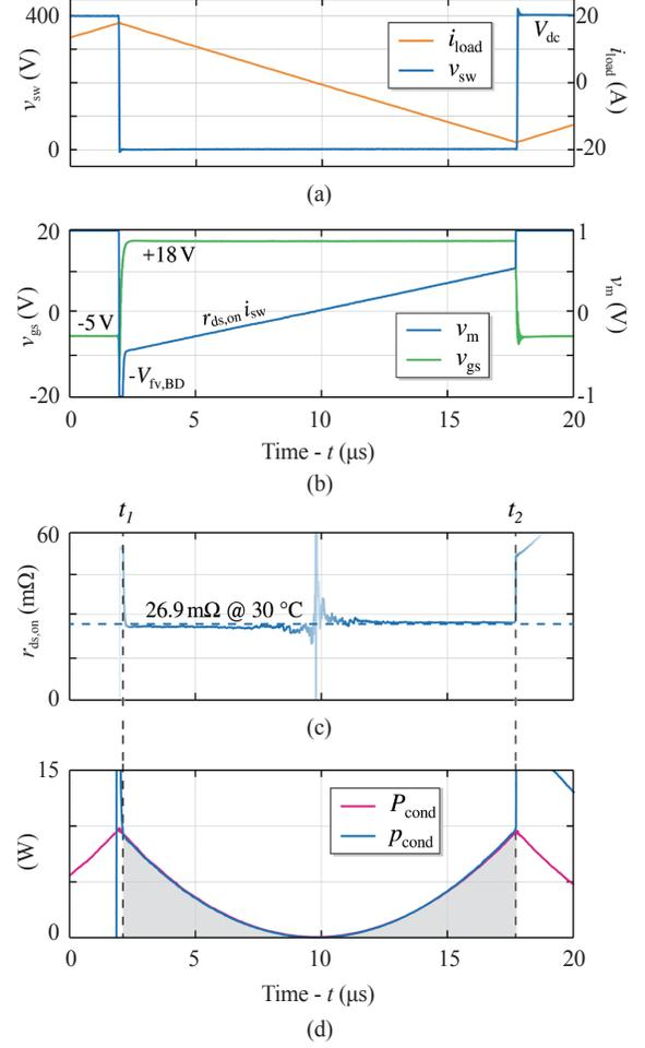
Fig. 11. Typical waveforms (a)-(b) measured on the half-bridge (Fig. 1) operating in triangular current mode (TCM). When  $v_{gs} = V_{gs,ON}$  (green),  $T_2$  conducts and  $v_m$  (blue) is proportional to  $i_{sw}$  (orange). In (c)  $r_{ds,on}$  is calculated between  $t_1$  and  $t_2$  dividing  $v_m$  by  $i_{sw}$ , while in (d)  $p_{cond}$  is obtained multiplying  $v_m$  and  $i_{sw}$ .
