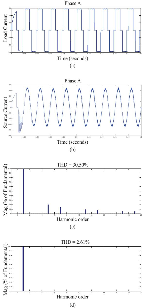
Fig. 9. (a) Balanced load current, (b) Phase-a source current after compensation after combination of load using VLLMS decomposer, (c) Harmonic analysis for load current, (d) Harmonic analysis for source current with VLLMS decomposer.
