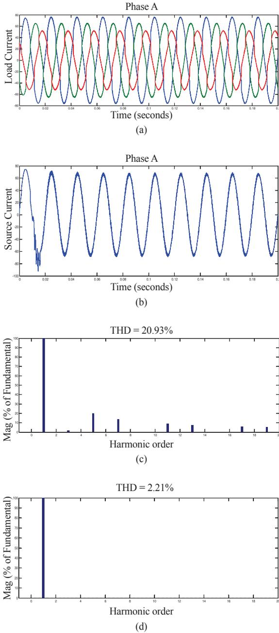
Fig. 8. (a) Unbalanced load current, (b) Phase-a source current after compensation after combination of load using VLLMS decomposer, (c) Harmonic analysis for load current, (d) Analysis for source current with VLLMS decomposer.
