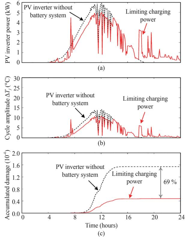
Fig. 10. Loading of PV the inverter with limiting charging power control strategy: (a) PV inverter power  $P_{pv}$ , (b) the thermal cycle amplitude of the power device  $\Delta T_j$ , and (c) the damage accumulation of the power device.
