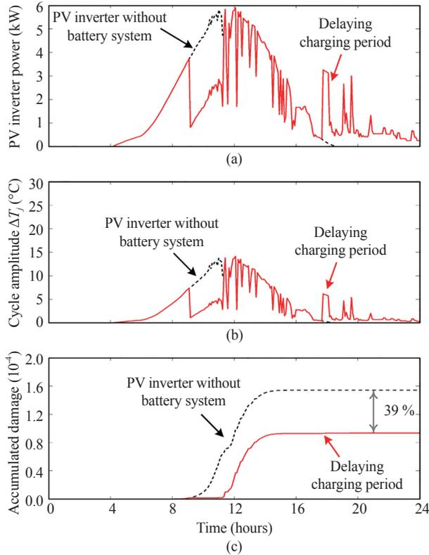
Fig. 9. Loading of the PV inverter with the delaying charging period control strategy: (a) PV inverter power  $P_{pv}$ , (b) the thermal cycle amplitude of the power device  $\Delta T_j$ , and (c) the damage accumulation of the power device.
