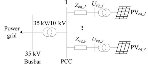
Fig. 4. Equivalent model of regional decentralized PV cluster.
