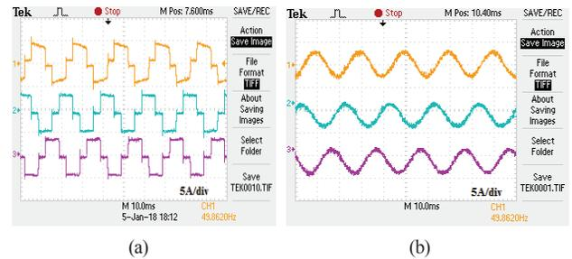
Fig. 14. Highly inductive load case (a) Load current, (b) Source current after compensation.
