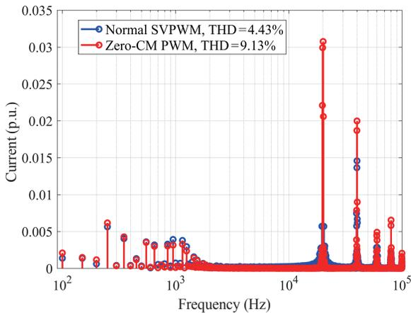
Fig. 19. Comparison of phase current spectrum: zero-CM PWM and normal SVPWM (experimental result).
