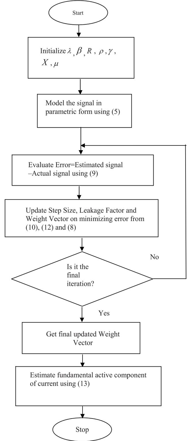
Fig. 2. Flow chart of the active fundamental current extraction scheme of VLLMS algorithm.
