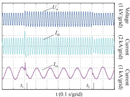
(b) Experimental waveforms for DFIG current and voltage when the grid voltage swelling to 130%.
