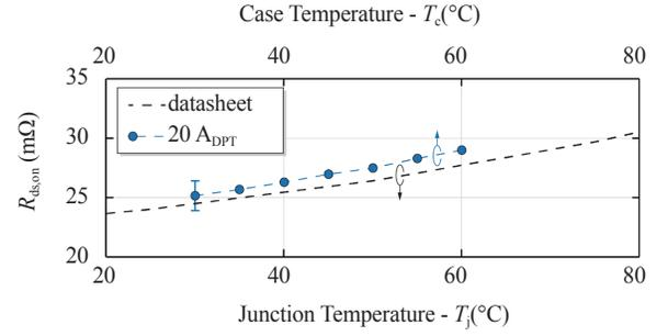
Fig. 13. Average value of  $r_{ds,on}$  (i.e.  $R_{DPT}$ ) measured with the proposed OVMC in double pulse test (DPT) operation for Specimen A in TABLE II compared with the nominal  $R_{ds,on}$  values reported in its datasheet (i.e.  $R_{data}$ ). The measured points match the nominal values within  $\pm 3\%$ .
