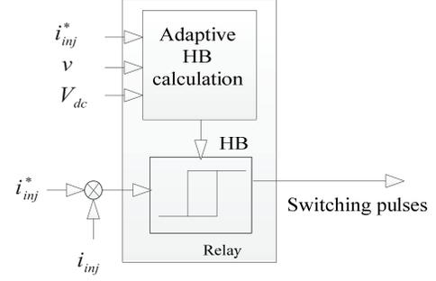
Fig. 4. Adaptive hysteresis band current controller.
