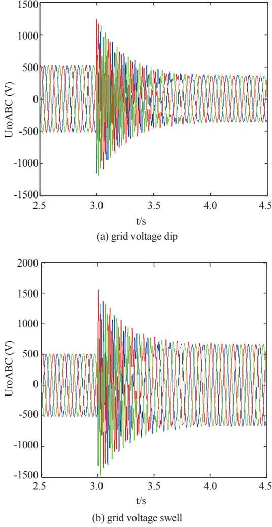
Fig. 3. Rotor three-phase open circuit voltage in grid fault.
