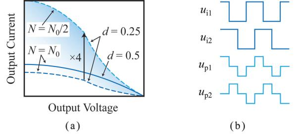
Fig. 6. (a) Reducing the duty cycle of the ISABC from 50% to 25% allows to reduce the number of turns by a factor of two, increasing the maximum output current. (b) Inverter voltages  $u_{i1}$ ,  $u_{i2}$  and winding voltages  $u_{p1}$ ,  $u_{p2}$  of the CISABC.
