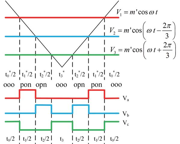
Fig. 23. Zero-CM SVPWM through carrier comparison.
