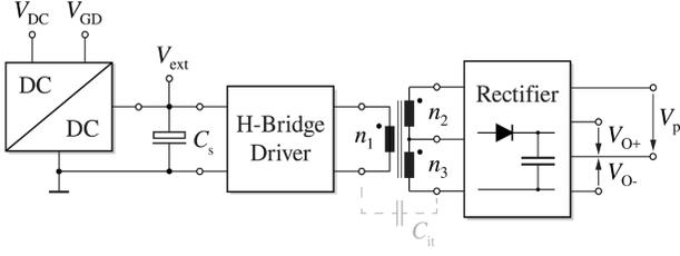
Fig. 5. Schematic representation of the OVMC supply circuitry.  $V_p$ ,  $V_{O+}$  and  $V_{O-}$  can be generated from one of the supply voltages available in the power converter, e.g.  $V_{DC}$  and  $V_{GD}$ , facilitating the integration of the OVMC. Galvanic isolation is guaranteed and a small value of parasitic capacitance  $C_{it}$  ensures high common-mode rejection ratio.
