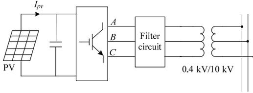
Fig. 2. The structure of a single PV system.
