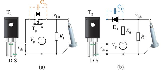
Fig. 2. Schematic representation of the two most common implementations of OVMCs. The input voltage  $v_{ds}$  is sensed at the DUT leads (see Fig. 1); by means of the MOSFET  $T_p$  (a) or of the diode  $D_1$  (b), the output is decoupled during the DUT off-state and connected during its on-state. While the dynamic performance of (a) are affected from  $C_{T_p}$ , the accuracy of (b) is compromised by  $v_{D_1}$ .
