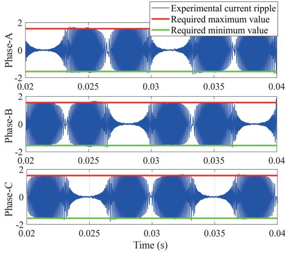
Fig. 27. Three-phase current ripple of zero-CM VSFPWM (experimental result).
