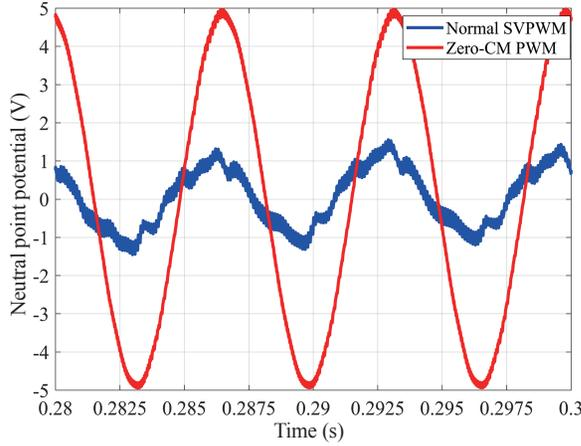
Fig. 22. Neutral point voltage comparison between normal SVPWM and zero-CM PWM.
