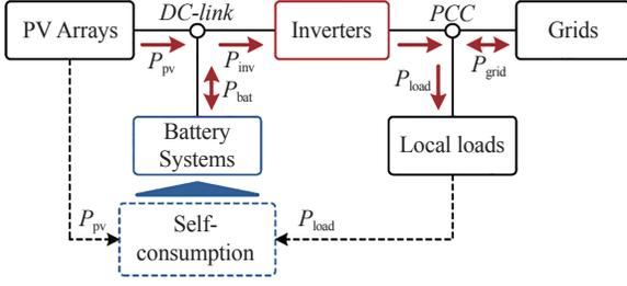
Fig. 1. Power flow of PV system with integrated battery system ( $P_{pv}$ : PV array output power,  $P_{bat}$ : battery power,  $P_{inv}$ : PV inverter input power,  $P_{load}$ : load consumption, and  $P_{grid}$ : power exchanged with the grid).
