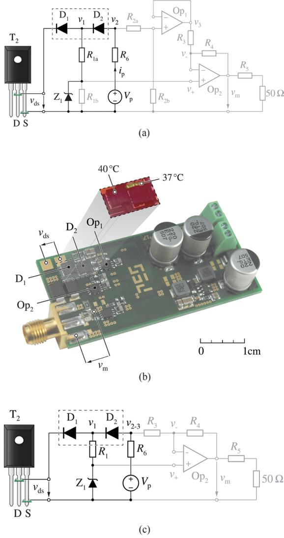
Fig. 4. Schematic representation of the realized (a) and simplified (c) versions of the proposed OVMC. (b) depicts the hardware realization of (a).  $D_1$  and  $D_2$  are thermally well coupled (dashed box) and electrically connected in series at the input of the OVMC in order to improve the measurement accuracy.
