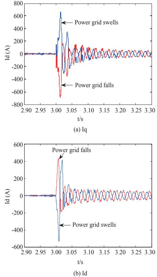
Fig. 8. Rotor current in dq frame of power grid swell and drop.
