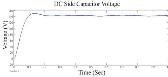
Fig. 6. Voltage of DC side capacitor in VLLMS based decomposer.
