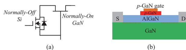
Fig. 1. Structure of GaN device: (a) Cascode GaN. (b) E-mode GaN.
