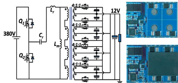
Fig. 16. Structure of integrated matrix transformer [77].
