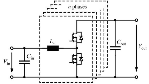
Fig. 2. Multi-phase boost converter.
