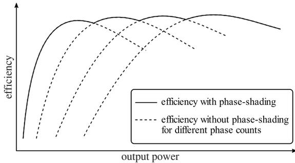
Fig. 3. Typical efficiency plot for multi-phase boost converters with and without phase-shading [14].
