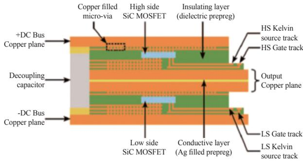
Fig. 9. CoC 3D power module structure [34].
