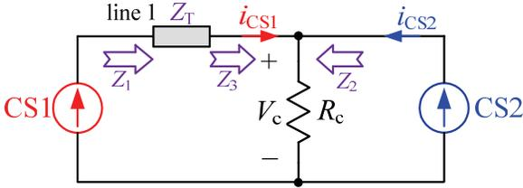
Fig. 7. Active load-pull technique.
