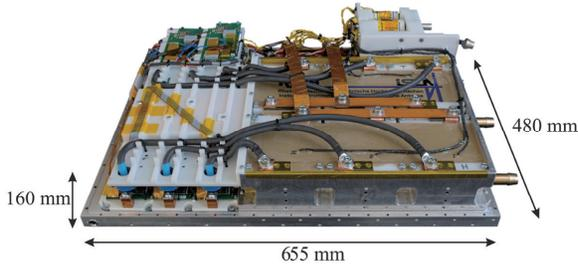
Fig. 6. 6-phase Si-based dc-dc converter with 240 kW peak power, 35 dm<sup>3</sup> displacement volume [23].
