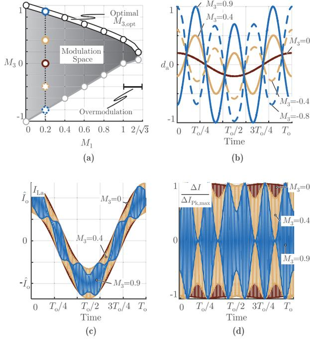
Fig. 4. Generalized third harmonic injection (GTHM) overview. In (a), the allowable  $M_3$  values depending on the modulation depth  $M_1$  are depicted. In (b), the effect of different values of  $M_3$  on the duty cycle of phase  $a$  for a constant modulation index  $M_1 = 0.2$  is visualized. In (c) and (d), the impact of the GTHM modulation technique on the inductor current and the current ripple is shown respectively.
