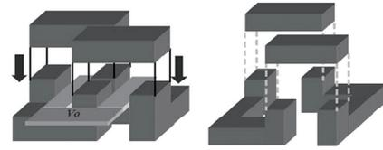
Fig. 14. Structure of the twisted core coupled inductor [73].
