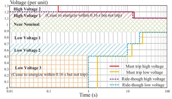
Fig. 10. Voltage ride-through requirements.
