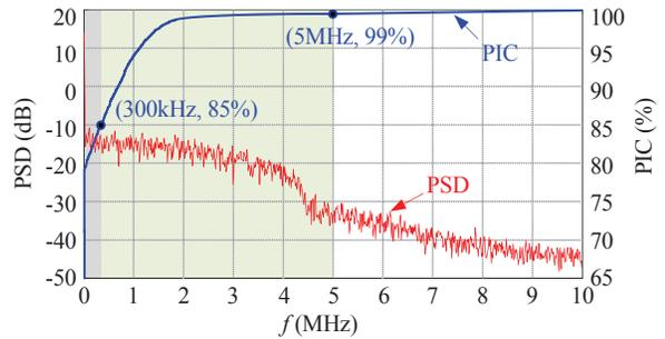
Fig. 17. PSD and PIC of the WCDMA envelope signal.
