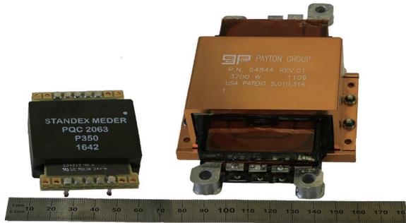
Fig. 16. Comparison of a 500 kHz transformer (left) and a 50 kHz transformer (right) for a power rating of 3.7 kW.
