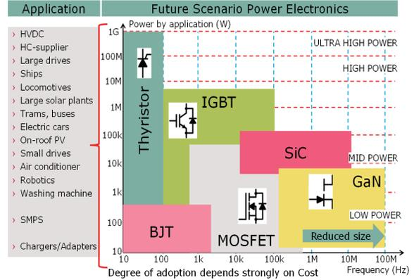
Fig. 6. Switching power device application space.
