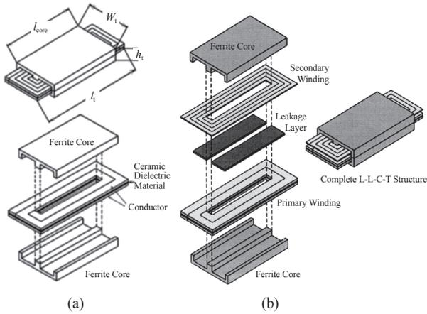
Fig. 17. Structure of LC and LLCT module [91].
