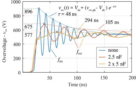
Fig. 5. Measured waveforms of the voltage across  $T_L$  during hard turn-on switching transition of  $T_H$  (i.e.  $R_g = 1.5 \Omega$ ,  $L_{ext} = 15 \text{ nH}$ ) with (red and yellow) and without (blue) integrated buffer capacitor  $C_b$ . A  $C_b$  bigger than 2.5 nF already significantly reduces the peak of  $v_{ov}$ , however, without a proper damping network, a prolonged oscillation occurs.
