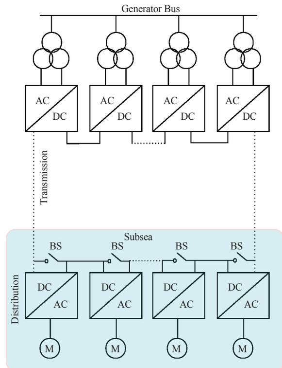
Fig. 3. Subsea modular stacked direct current structure [8].
