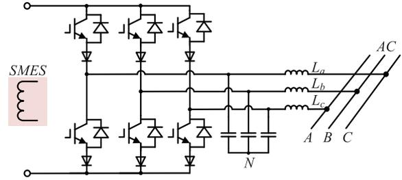
Fig. 22. Three-phase current source inverter.
