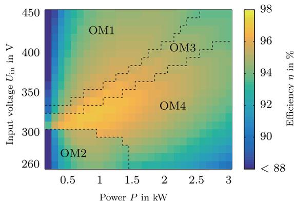
Fig. 10. Efficiency of a three-phase dual-active bridge converter using optimized operation strategies (simulation results).
