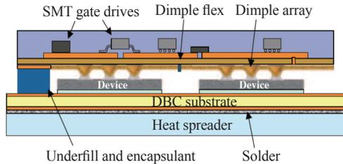
Fig. 4. DAI based module structure [20].
