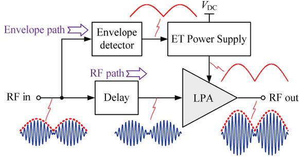
Fig. 9. Scheme diagram and key waveforms of ET technique.
