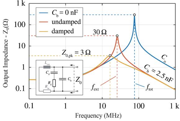
Fig. 7. Output impedance of the  $C_b$ - $R_dC_d$  network ( $Z_0$ ) for  $C_b = 2.5$  nF with (yellow) and without (red) the damping network. The optimized damping network ( $R_d = 1.5$   $\Omega$  and  $C_d = 5$  nF) reduces  $Z_{0,pk}$  from 30  $\Omega$  to 3  $\Omega$  according to the specifications. The impedance without  $C_b$  seen from the AC terminal is also plotted (blue) to highlight the shifting of the main resonance from  $f_{tot}$  to  $f_{ext}$ .
