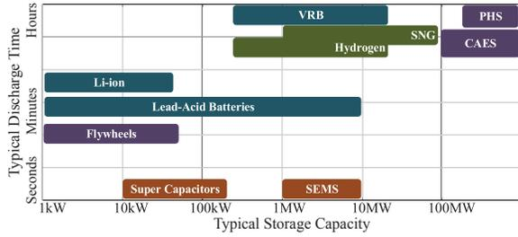
Fig. 4. Typical power capacity and discharge time for ESSs.
