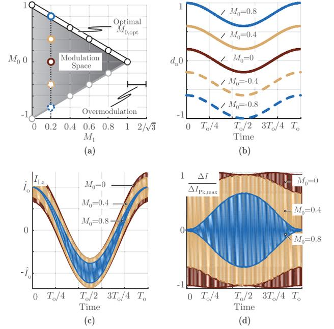
Fig. 3. Constant CM shifting (DCCMM) overview. In (a), the available  $M_0$  values depending on the modulation depth  $M_1$  are depicted. In (b), the effect of different values of  $M_0$  on the duty cycle of phase  $a$  for a constant modulation index  $M_1 = 0.2$  is visualized. In (c) and (d), the impact of the DCCMM modulation technique on the inductor current and the current ripple is shown respectively.
