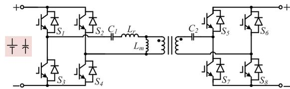
Fig. 19. CLLC DC/DC converter.
