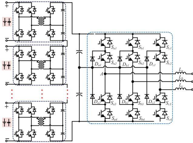
Fig. 25. Series DC bus configuration.
