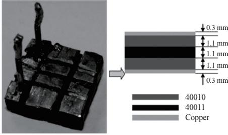
Fig. 28. Prototype of the nonlinear LTCC inductor [125].
