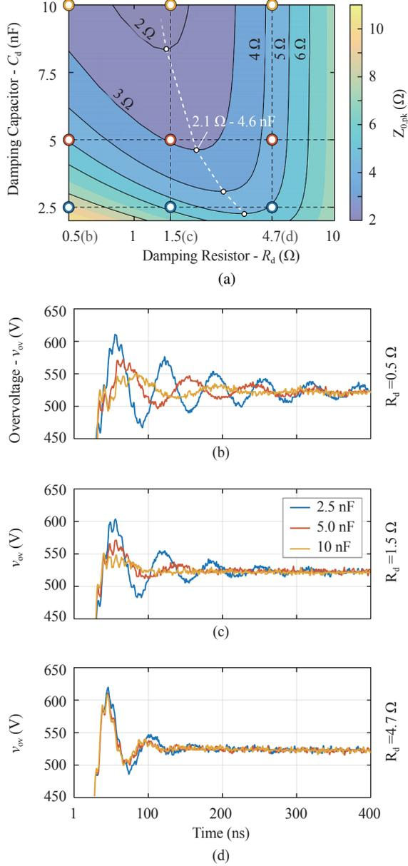
Fig. 8. Peak of the output impedance of the buffer-damping network ( $Z_{0,pk}$ ) for  $0.5 \Omega < R_d < 10 \Omega$  and  $2 \text{ nF} < C_d < 10 \text{ nF}$  (a). The colored dots highlight the combinations of  $R_d$  and  $C_d$  whose associated  $v_{ov}$  measured waveforms are shown in (b), (c) and (d). Finally, the white dashed line represents the locus of the optimum designs according to [33].  $C_b$  is fixed to 2.5 nF,  $L_{ext}$  to 15 nH and  $R_{ac}$  to 200 m $\Omega$ .
