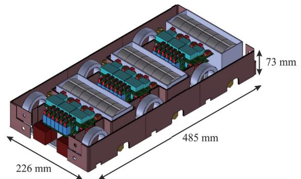
Fig. 5. CAD-model of a 9-phase SiC-based buck-boost converter consisting of 3 converter building blocks, resulting in 126 kW peak power.
