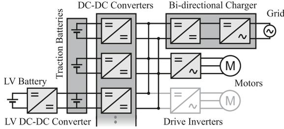
Fig. 1. Modular propulsion system architecture.
