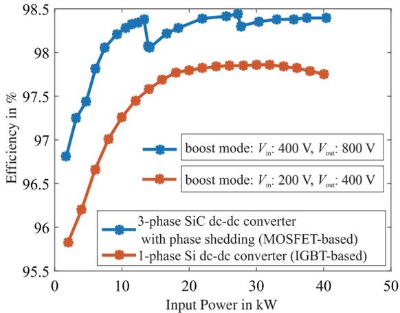
Fig. 7. Efficiency comparison of the 3-phase interleaved SiC converter building block and 1 phase of the 6-phase Si dc-dc converter.
