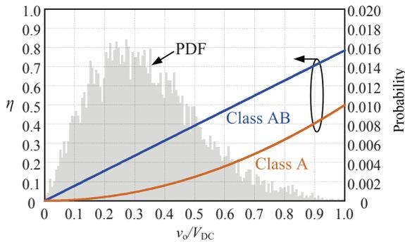
Fig. 13. Efficiency curves of the linear amplifiers and PDF of the envelope signal versus normalized output voltage.
