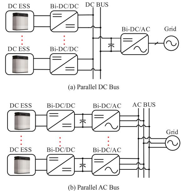
Fig. 24. Parallel DC and AC bus structures.
