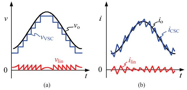
Fig. 21. Key waveforms of series-parallel-form SLH ET power supply. (a) Key voltage waveforms. (b) Key current waveforms.
