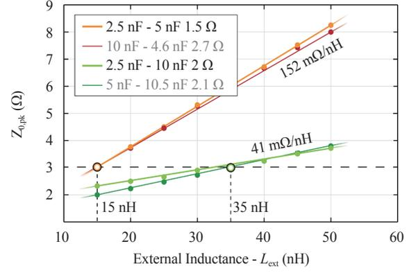
Fig. 9. Sensitivity of  $Z_b$ , representing the figure of merit of the  $C_b$ - $R_d$  $C_d$  network, towards  $L_{ext}$  for different [33]-optimized combinations. When the network is designed ( $Z_{0,pk} = 3 \Omega$ ) for 15 nH (orange and red), the required overall capacitance is less than in the case of 35 nH (light and dark green), however the sensitivity is almost four times higher.
