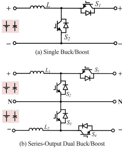
Fig. 16. Bidirectional buck/boost converter.
