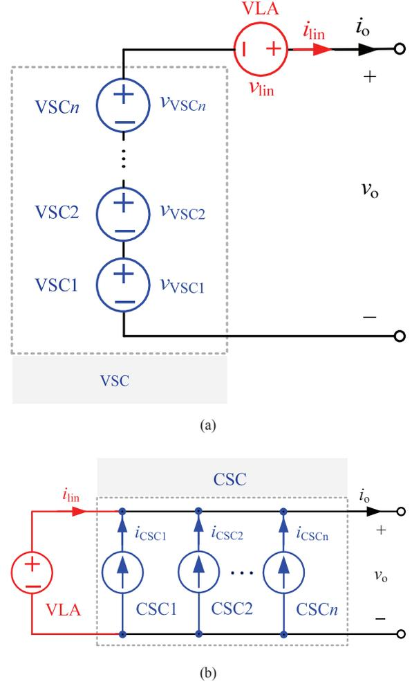
Fig. 26. SLH structures with multiple switched-mode converters. (a) Series-form SLH structure with multiple VSCs. (b) Parallel-form SLH structure with multiple CSCs.
