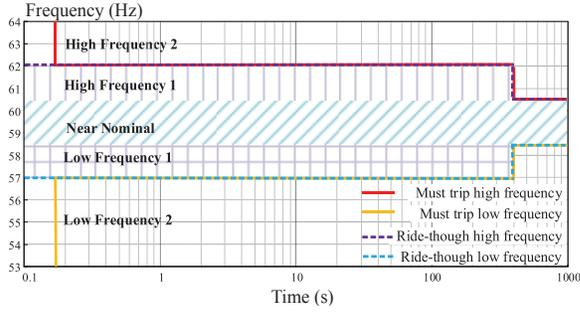
Fig. 11. Frequency-ride through requirements.
