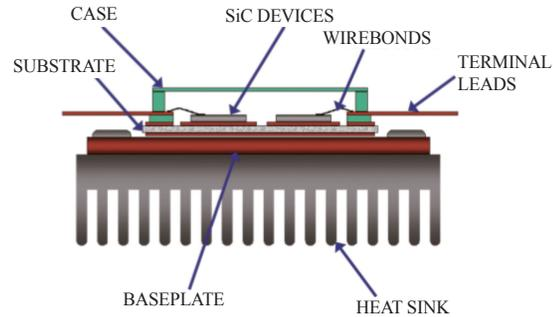
Fig. 1. Conventional wire-bonding power module structure [37].
