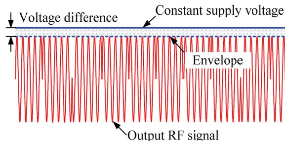
Fig. 1. Key waveforms of the LPA in 2G mobile communication system.
