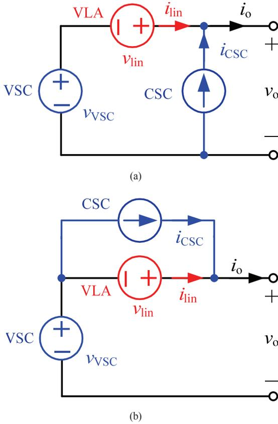
Fig. 20. Block diagram of series-parallel-form SLH ET power supply. (a) Type I. (b) Type II.
