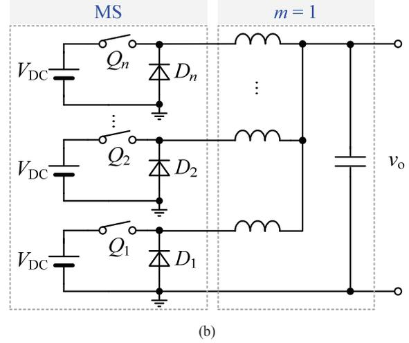
Fig. 16. Schematic diagrams of typical MS structures. (a) Multilevel MS. (b) Multiphase MS.
