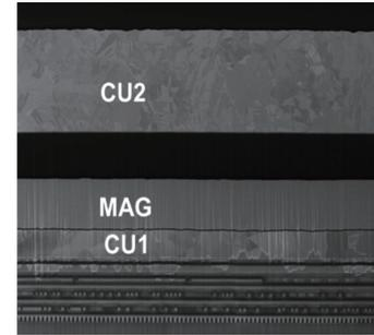
Fig. 9. SEM cross section of magnetic thin-film inductors integrated with CMOS IC.
