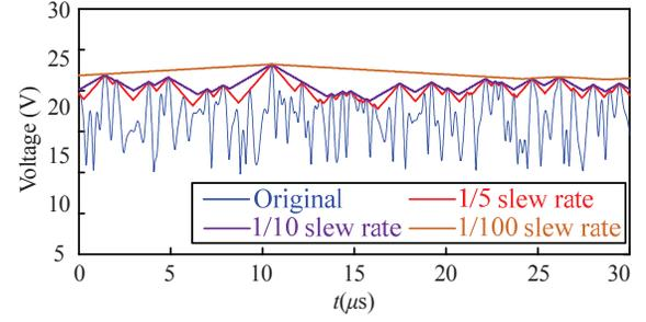
Fig. 23. Envelope signals with different slew rate.
