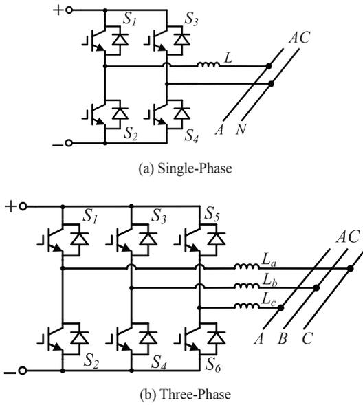
Fig. 20. Bidirectional two-level DC-AC converter.
