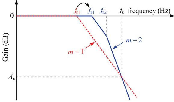
Fig. 15. Gain curves versus frequency of the single-stage and two-stage filters.
