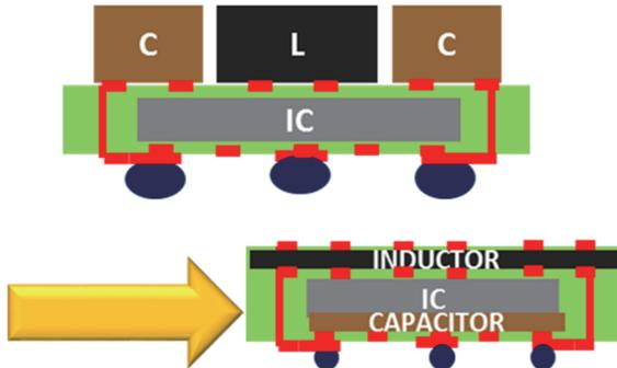
Fig. 8. Embedding of capacitor and inductor (Courtesy of Georgia Tech).
