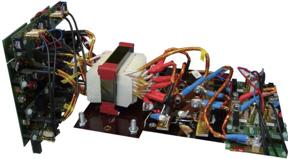
Fig. 13. Photograph of a 10 kW laboratory prototype of a single-phase dual-active bridge converter with tap changer [38].
