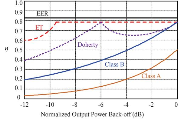
Fig. 11. Efficiency curves of power amplifiers using different techniques versus normalized output power back-off.
