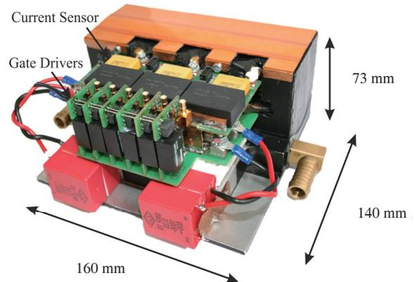
Fig. 4. 3-phase SiC-based boost converter prototype without copper bus-bars and common mode chokes.
