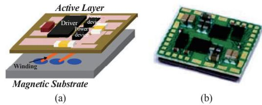
Fig. 27. 3D integration POL converter [115]. (a) Schematic. (b) Prototype of a two-phase interleaved converter.
