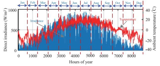
Fig. 2. Yearly direct irradiance and ambient temperature data of the site with hourly intervals.
