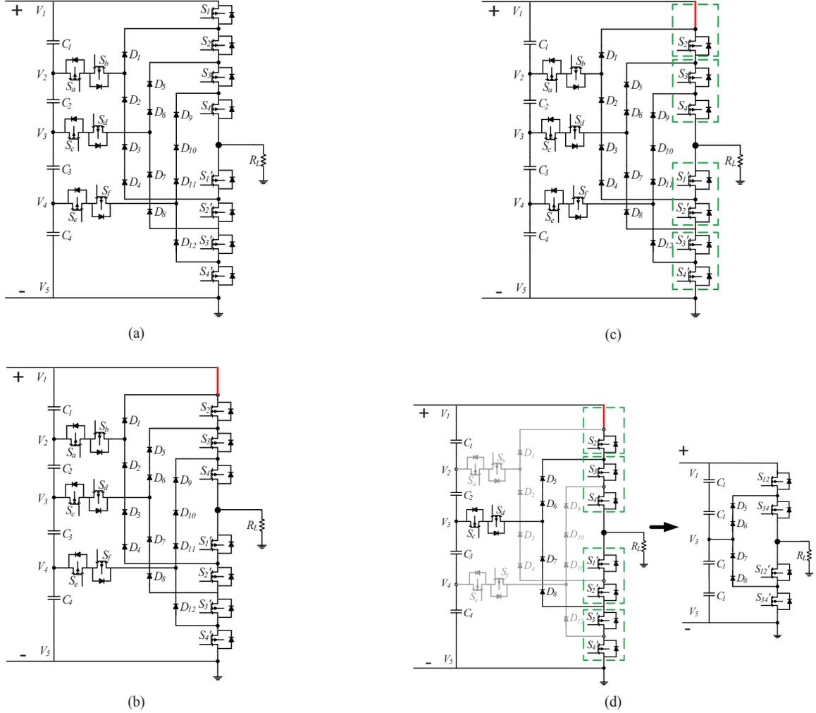
Fig. 4. Proposed topology (a) Healthy condition, (b) Short circuit fault in  $S_1$ , (c) Switching in pairs, (d) Fully reconfigured condition with turning off back-to-back switches  $S_{1a}$ ,  $S_{1b}$ ,  $S_{1c}$  and  $S_{1d}$ .
