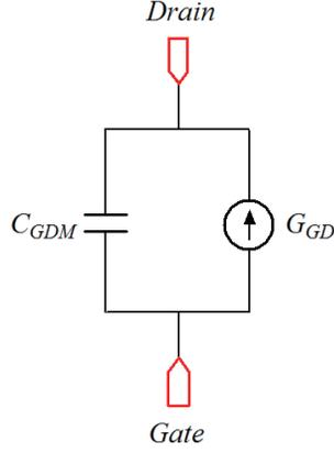
Fig. 3. Simplified  $C_{GD}$  model in this work.
