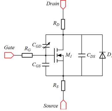
Fig. 2. Proposed SPICE sub-circuit model of SiC MOSFET in this work.
