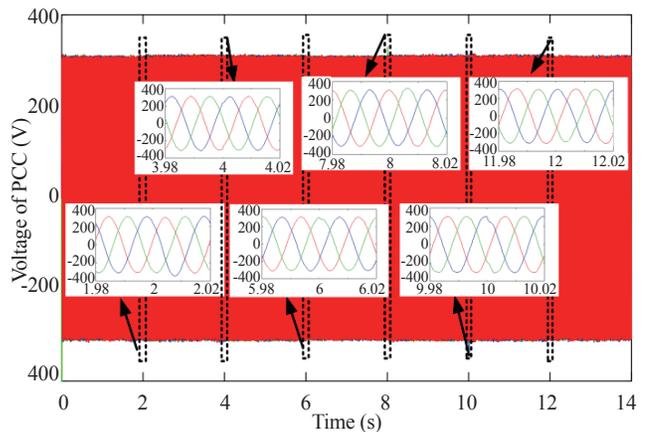
Fig. 14. PCC voltage corresponding to changes of insolation.
