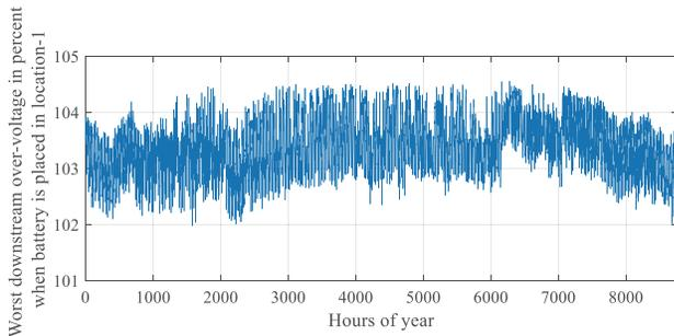
Fig. 12. Worst downstream over-voltage when the BESS is placed in location #1.
