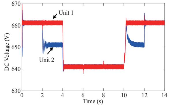
Fig. 13. DC voltages corresponding to changes of insolation.
