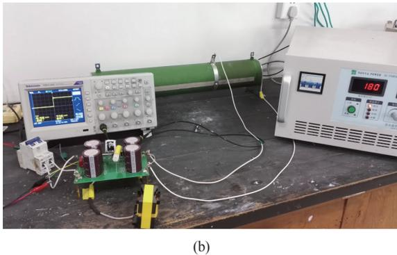
Fig. 7. Schematic of Boost converter in LTspice IV (a) and the experimental platform (b).
