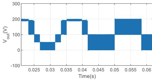
Fig. 10. Output waveform of transmitting  $S_1$  short circuit condition to re-configured condition.
