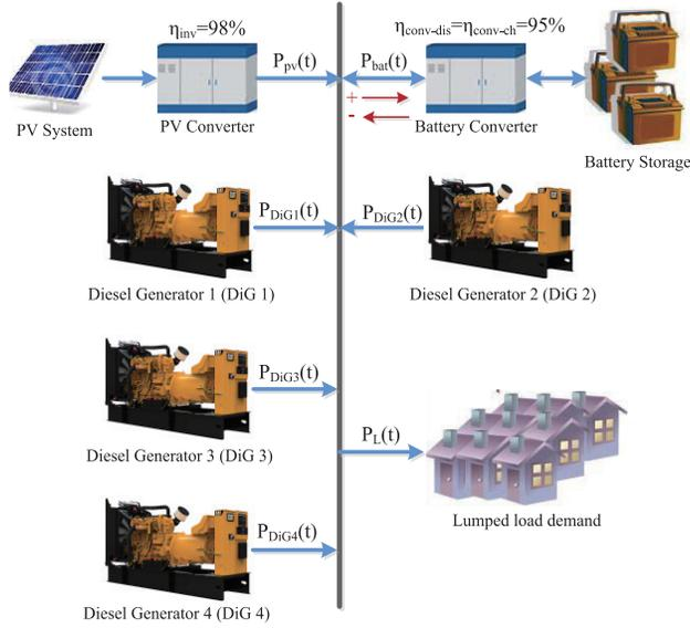
Fig. 1. Simplified configuration of the desired hybrid PV/BESS/DiGs microgrid on a remote site in Northern Canada.
