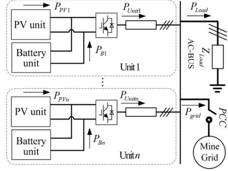
Fig. 1. Structure diagram of the researched microgrid.
