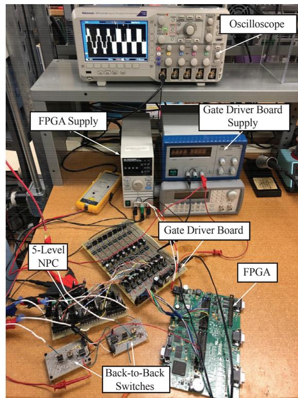
Fig. 13. Hardware Setup.
