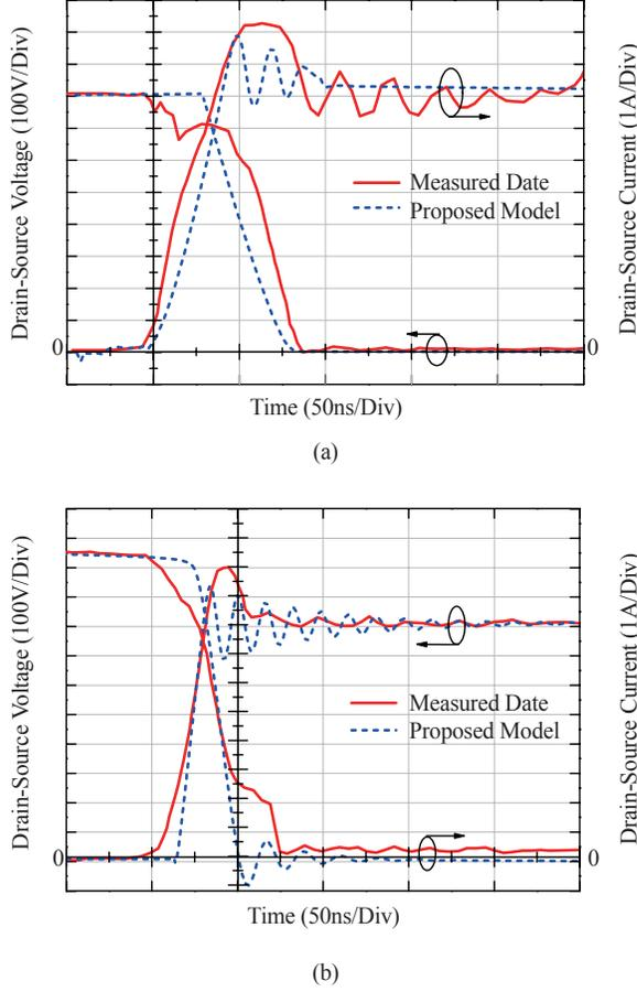
Fig. 9. Comparison of turn-on (a) and turn-off (b) waveforms at 800 V between LTSpice IV simulation and experiment in Boost converter.
