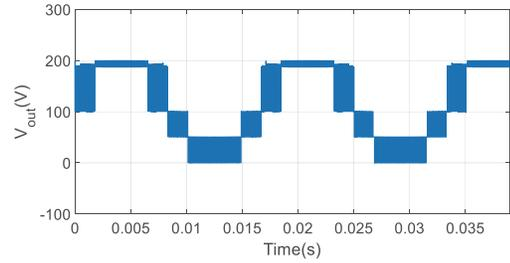
Fig. 8. Output waveform of  $S_i$  short circuit fault.
