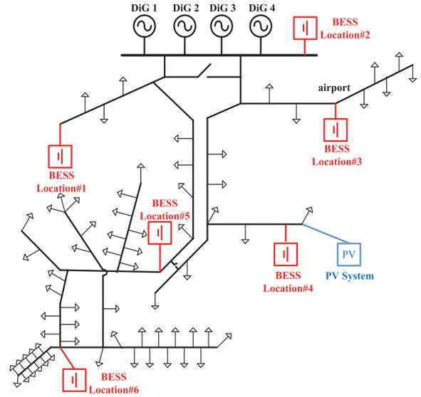
Fig. 10. Simplified schematic of the case study site in Northern Canada and the six selected locations for the BESS installation.
