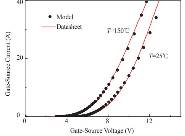
Fig. 5. Comparison of transfer characteristics between this developed SPICE model with C2M0080120D Datasheet.
