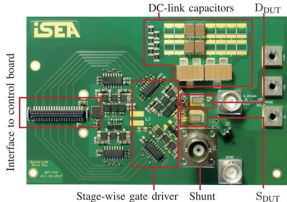
Fig. 4. Photograph of the PCB containing the driver and SiC bare dies.
