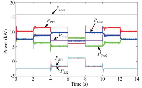
Fig. 12. Output powers of each unit corresponding to changes of insolation.
