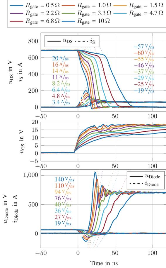
Fig. 10. Reference turn-on event measurements using different gate resistors.
