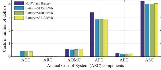
Fig. 8. Different elements of the ASC under optimal PV and battery size.
