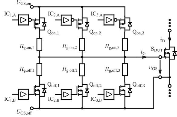
Fig. 1. Topology of the proposed stage-wise driver.
