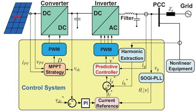
Fig. 6. Control structure of PV systems for harmonic compensation.
