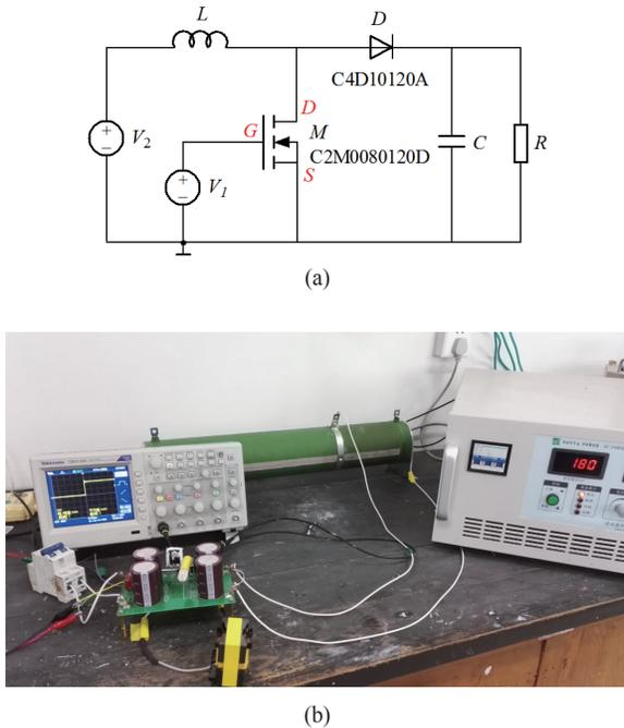
Fig. 7. Schematic of Boost converter in LTspice IV (a) and the experimental platform (b).
