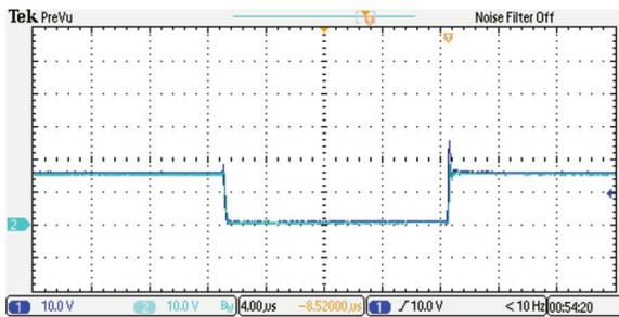
Fig. 17. Balanced condition of  $S_1$  and  $S_2$  voltage (10 V/div, 4  $\mu$ s/div).
