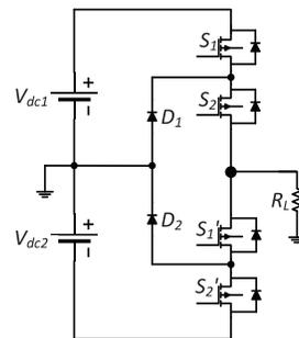
Fig. 1. Single Phase of a Three-level NPC.
