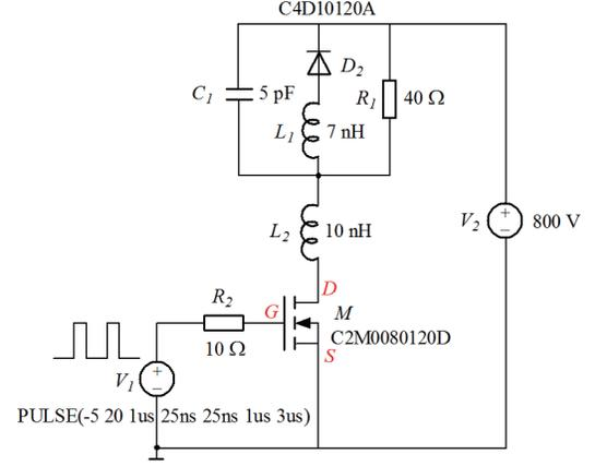
Fig. 10. Clamped inductive switching circuit for simulation of SiC MOSFET's switching loss.
