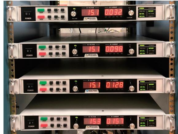
Fig. 12. Isolated power supplies.
