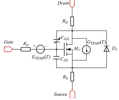
Fig. 1. SPICE sub-circuit model of SiC MOSFET in [11] and [12].
