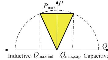
Fig. 3. 2-quadrant  $P$ - $Q$  control method.
