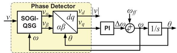
Fig. 9. The structure of SOGI-PLL.
