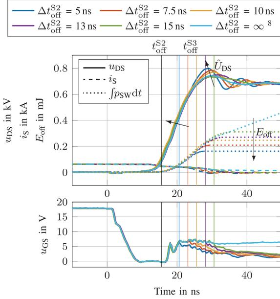
Fig. 17. Three-stage turn-off event waveforms.
