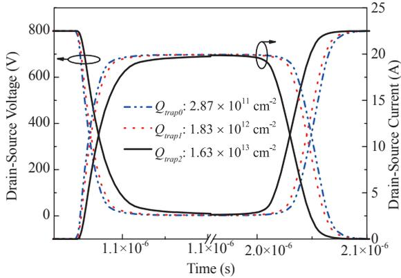
Fig. 12. Switching waveforms of SiC MOSFET for different  $Q_{trap}$ .
