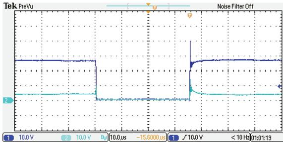
Fig. 16. Unbalanced condition of  $S_1$  and  $S_2$  voltage (10 V/div, 10  $\mu$ s/div).
