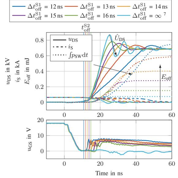
Fig. 16. Two-stage turn-off event waveforms using  $R_{g,\text{off}}^{S2} = 15 \Omega$ .TABLE VIII
