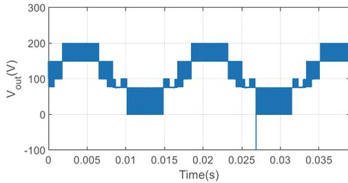
Fig. 9. Output waveform of  $S_3$  short circuit fault.
