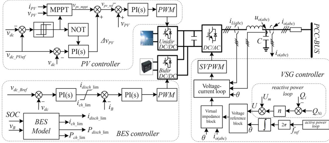
Fig. 2. Control structure of the proposed control strategy.
