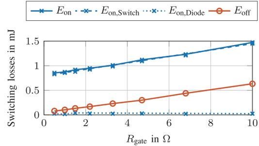
Fig. 12. Calculated switching losses using the reference driver with various gate resistances at  $U_{\text{dc}} = 700 \text{ V}$ ,  $I_{\text{D}} = 60 \text{ A}$ .
