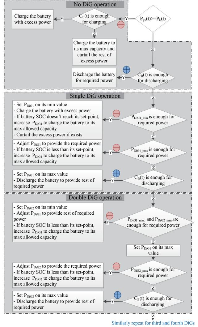
Fig. 3. Flowchart of dispatch strategy of the hybrid PV/BESS/DiGs microgrid.
