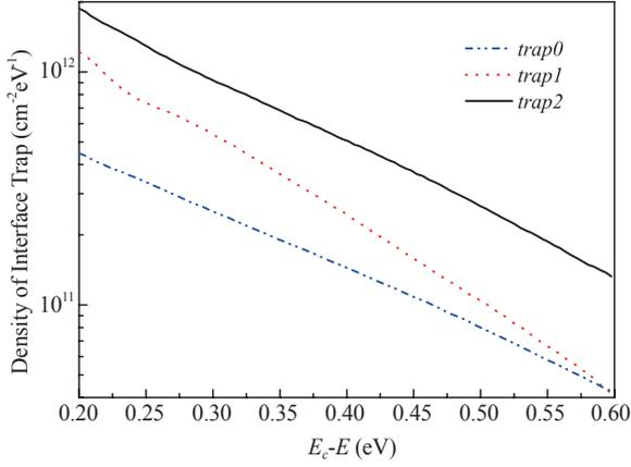
Fig. 11. Three distributions of interface traps for LTspice simulation [29].
