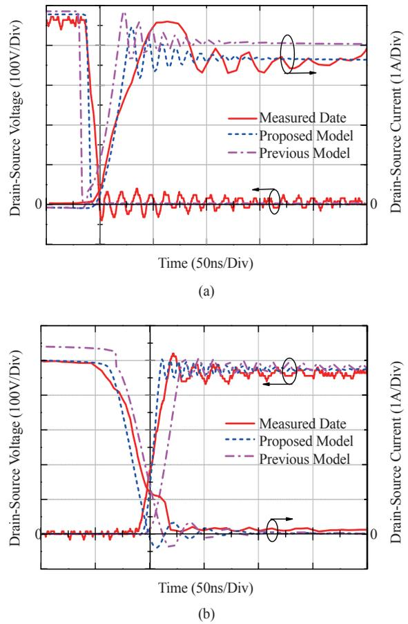
Fig. 8. Comparison of turn-on (a) and turn-off (b) waveforms at 470 V between LTspice IV simulation and experiment in Boost converter.
