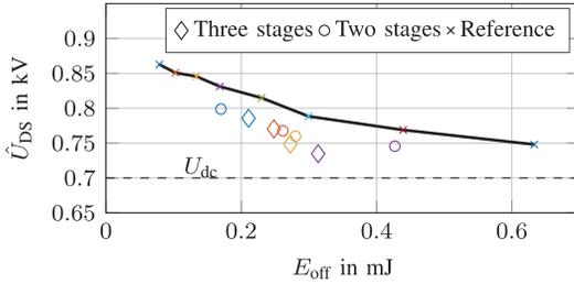
Fig. 18. Low-side switch voltage overshoot vs. turn-off energy.
