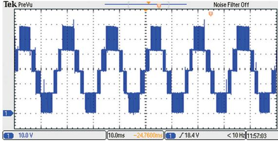
Fig. 14. Healthy operation with 200 V DC bus (10 V/div, 10 ms/div).
