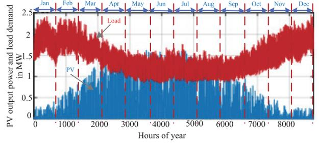
Fig. 6. Yearly load demand and PV system power production on the site.
