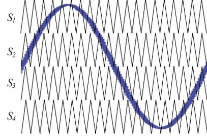
Fig. 3. Level shifted PWM for five-level NPC.
