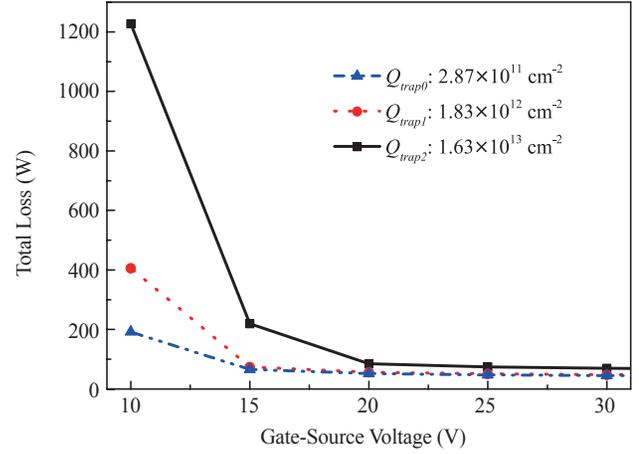
Fig. 13. Relationship between gate voltage and the total loss of SiC MOSFET with different interface traps.
