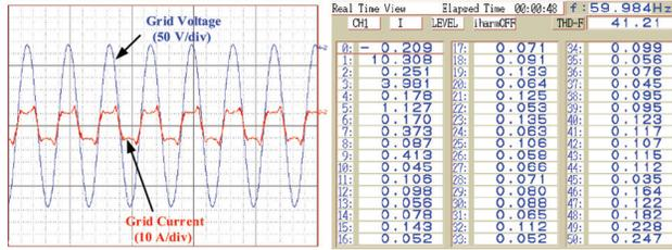
(a) PCC current waveform and harmonics, without compensation
