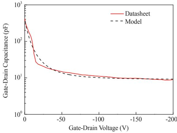
Fig. 4. Comparison of  $C_{GD}$  between a simplified model and C2M0080120D Datasheet.
