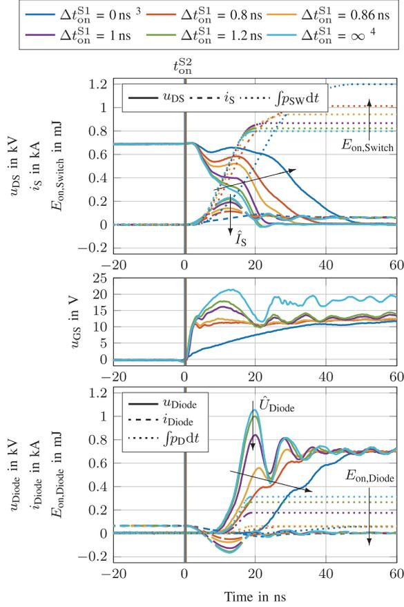
Fig. 13. Two-stage turn-on event waveforms using  $R_{g,on}^{S2} = 10 \Omega$ .
