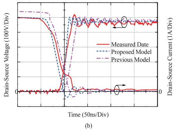
Fig. 8. Comparison of turn-on (a) and turn-off (b) waveforms at 470 V between LTspice IV simulation and experiment in Boost converter.
