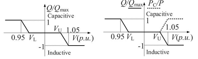
(a)  $Q(V)$  control method(b)  $Q(V)/P(V)$  control method
