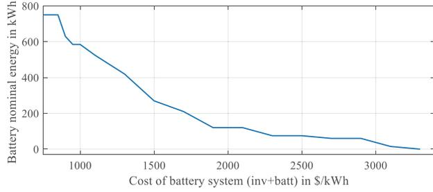
Fig. 9. Optimal size of the BESS under different battery bank costs.
