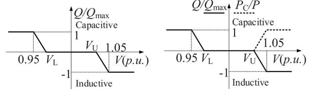
(a)  $Q(V)$  control method(b)  $Q(V)/P(V)$  control method
