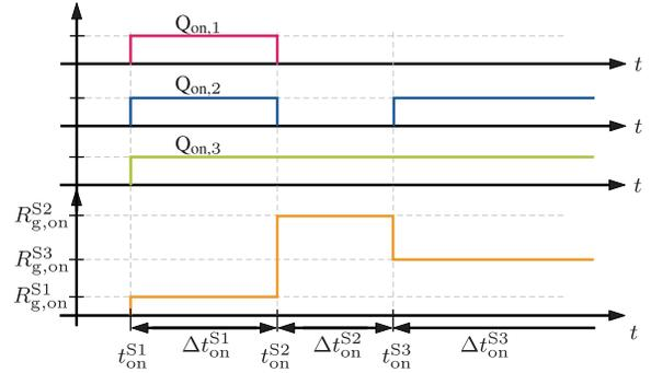
Fig. 2. Operation principle of the stage-wise driver.
