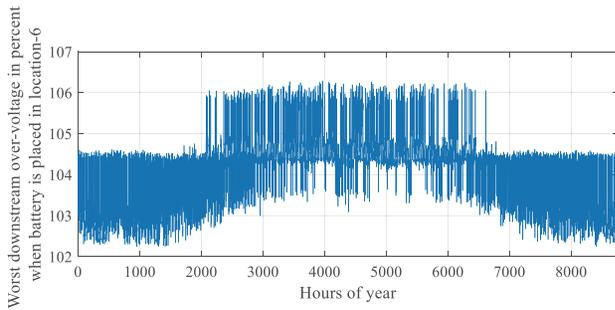
Fig. 11. Worst downstream over-voltage when the BESS is placed in location #6.
