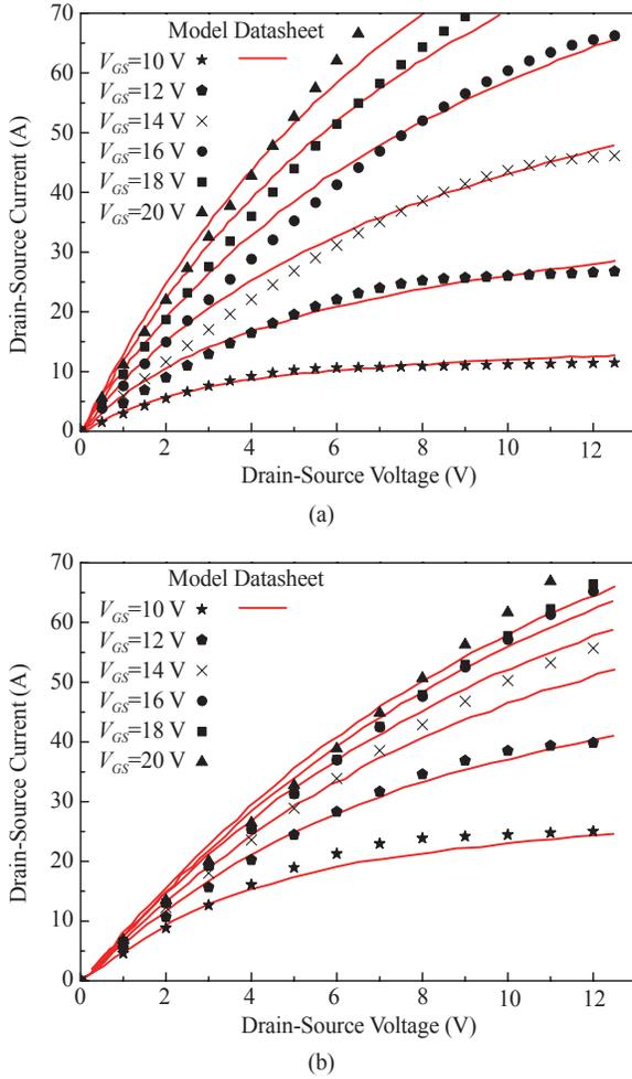
Fig. 6. Comparison of output characteristics between this developed SPICE model with C2M0080120D Datasheet at  $25\text{ }^\circ\text{C}$  (a) and  $150\text{ }^\circ\text{C}$  (b).
