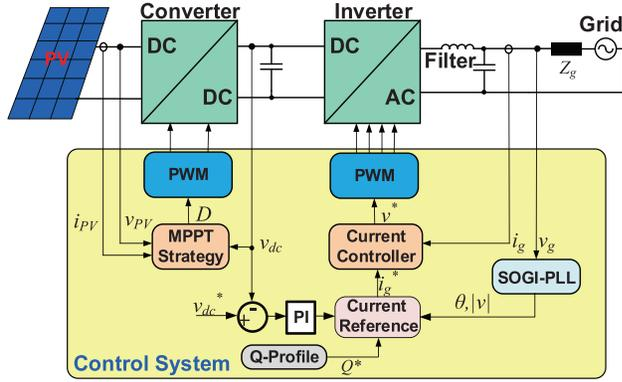
Fig. 4. Schematic diagram of single-phase grid-connected PV system.
