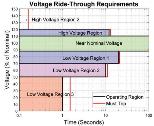
Fig. 8. Voltage ride-through regions according to Rule 21.
