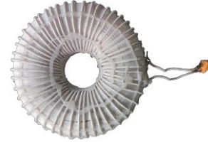
Fig. 11. Optimized air-core inductor (24.6 \mu H) for improved calibration accuracy.
