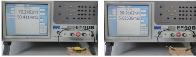
Fig. 24. Measurement diagram of (a) entire resistance and (b) lead resistance.
